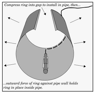
Figure 2-21 Sensor Installed on a Spring Ring
